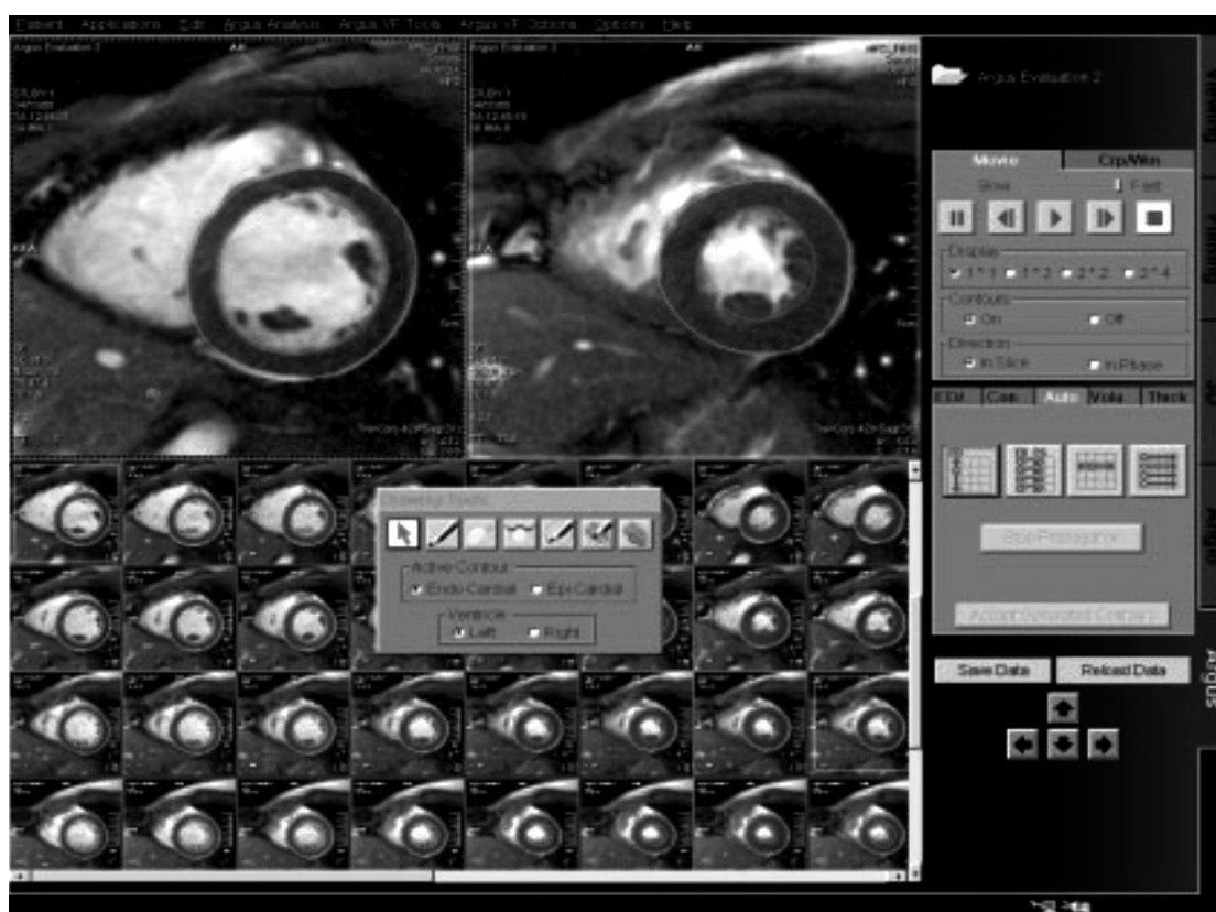
Figure 1 CMR diagnostic console with Siemens Argus software, to determine endo and epicardial contour left ventricular in enddiastolic and endsystolic phase in short axis. (Figure from the IZD archive in Trnava).
